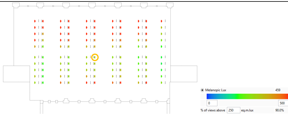
Figure 9 – Model 1. Melanopic Lux performance at 9 am, March 21 st . The yellow circle indicates the lowest illuminance.
