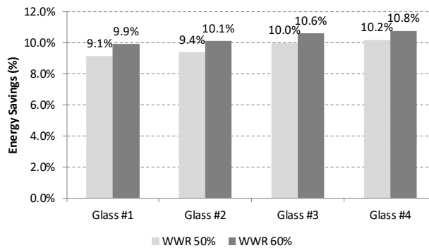
Figure 8 – Energy savings for cases with different glass types and WWR.
