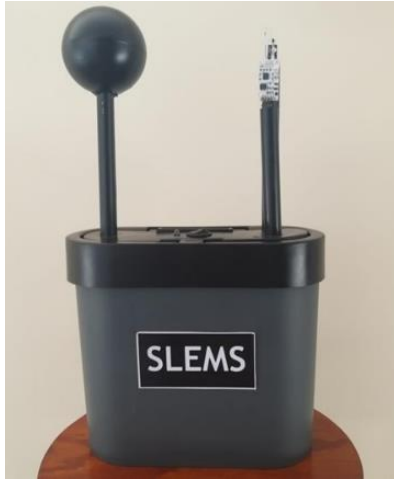
Figura 1– SLEMS (Stationary Low-cost Environmental Monitoring System).
