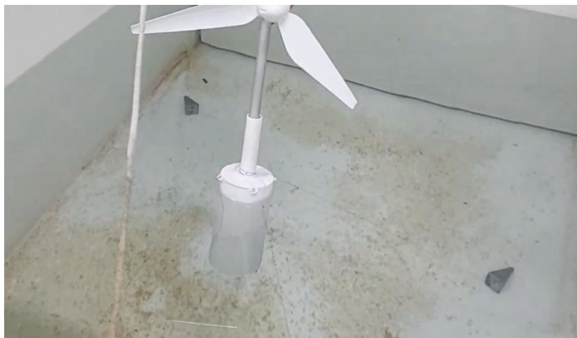
Figure 5 - Buoyancy test of Part 3 in the laboratory tank.
