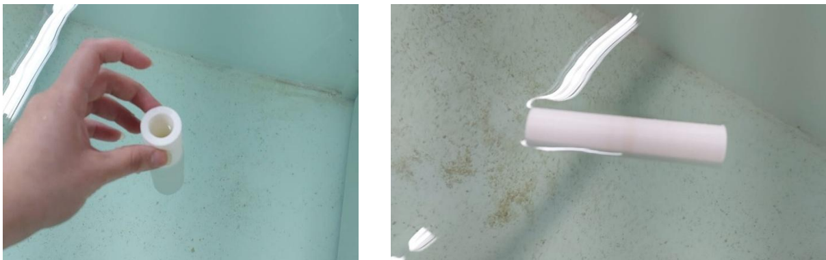
Figures 2a and 2b - Buoyancy test of the prototype in the laboratory tank.
