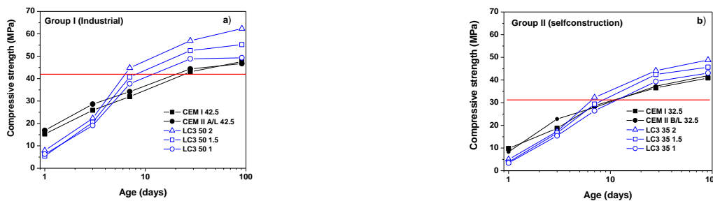
Fig. 1. Compressive strength of cements at 1, 3, 7, 28 and 91 days. a) Industrial segment; b) Self construction segment.
