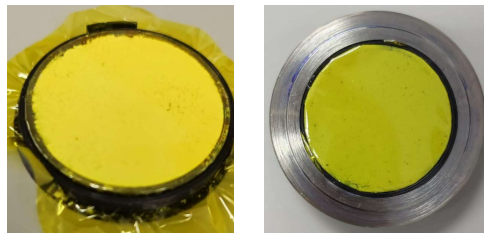
Figure 1: C-S-H pastes placed in the sample holder with Kapton film
